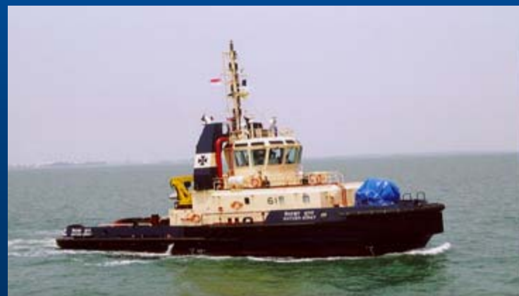
60 Ton Bollard Pull Azimuth Stern Drive Tug
