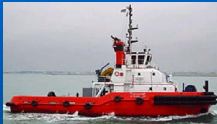
46 Ton Bollard Pull Azimuth Stern Drive Tug
